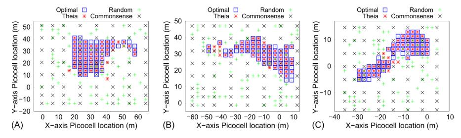
• Theia performs close to Optimal when placing picocells in outdoor environments
