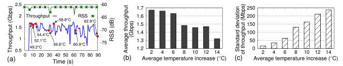
Figure 4: Link performance is affected by higher antenna temperature: (a) Link RSS is stable, but throughput fluctuates over time; every time index is marked for  $2^{\circ}C$  temperature increase; For every  $2^{\circ}C$  increase, we see changes in (b) Average throughput; and (c) Standard deviation of throughput.
