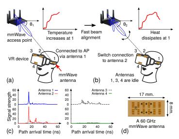
Figure 1: Core idea behind Aquilo: (a) VR device with 4 mmWave antennas connected to the access point (AP) via antenna 1; data transfer increases its temperature; (b) Scheduler switches to relatively cooler antenna 2 with the best link to the AP; (c) Signal strength of the best beam from the 4 antennas; (d) Dimensions of a 60 GHz mmWave antenna [8].
