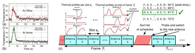
Figure 7: Data transfer for 10 s., and then, heat dissipation: (a) At office; and (b) At home. (c) Aquilo schedules antennas at the beginning of every frame  $\mathcal{F}_i$ ; then, probes and switches to a new antenna every slot  $s_k$ .
