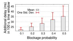
Figure 10: Delay under Aquilo within a window of 100 s. under different environmental conditions. The Error bar shows one standard deviation. The average overhead is less than 0.04%.
