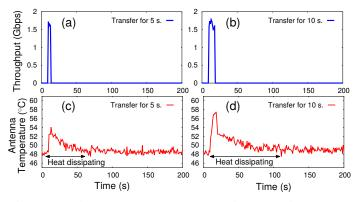
Figure 3: (*a–b*) Data transfers for 5 s. and 10 s. (*c–d*) Antenna temperatures over time and heat dissipation durations.
