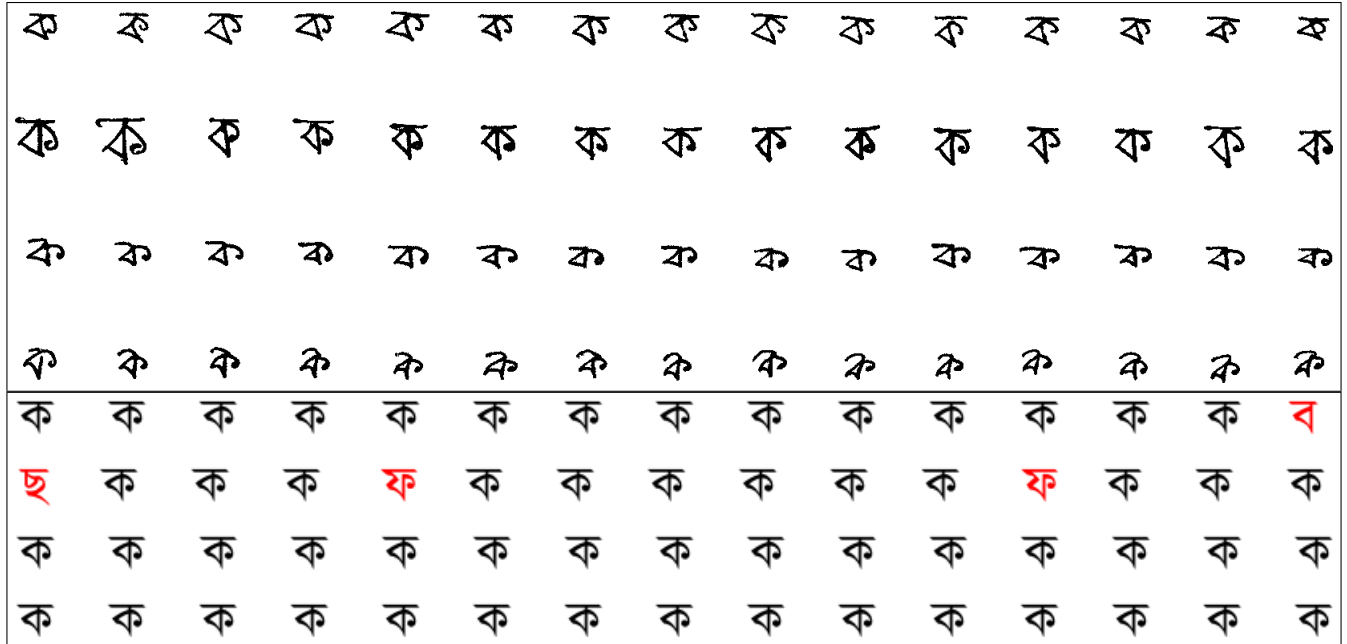
Figure 6. Top: Sample test images of ‘ka’ (the first Bangla consonant). Bottom: Recognition by Scheme 1; 36 out of 40 characters here are rightly classified, and 4 characters misclassified (15th, 16th, 20th, and 27th; shown in red).
