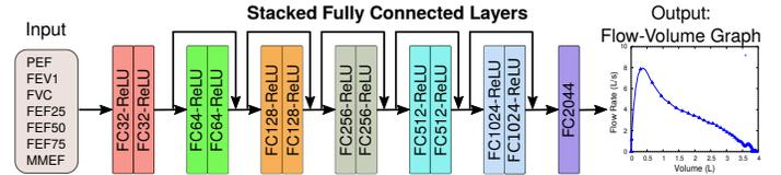
Figure 8: Deep residual decoder of the *mmFlow* system.
