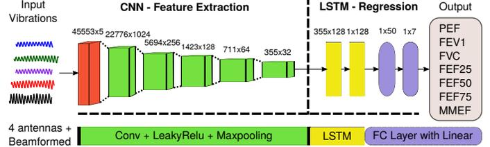
Figure 6: CNN-LSTM architecture of the *mmFlow* system.
